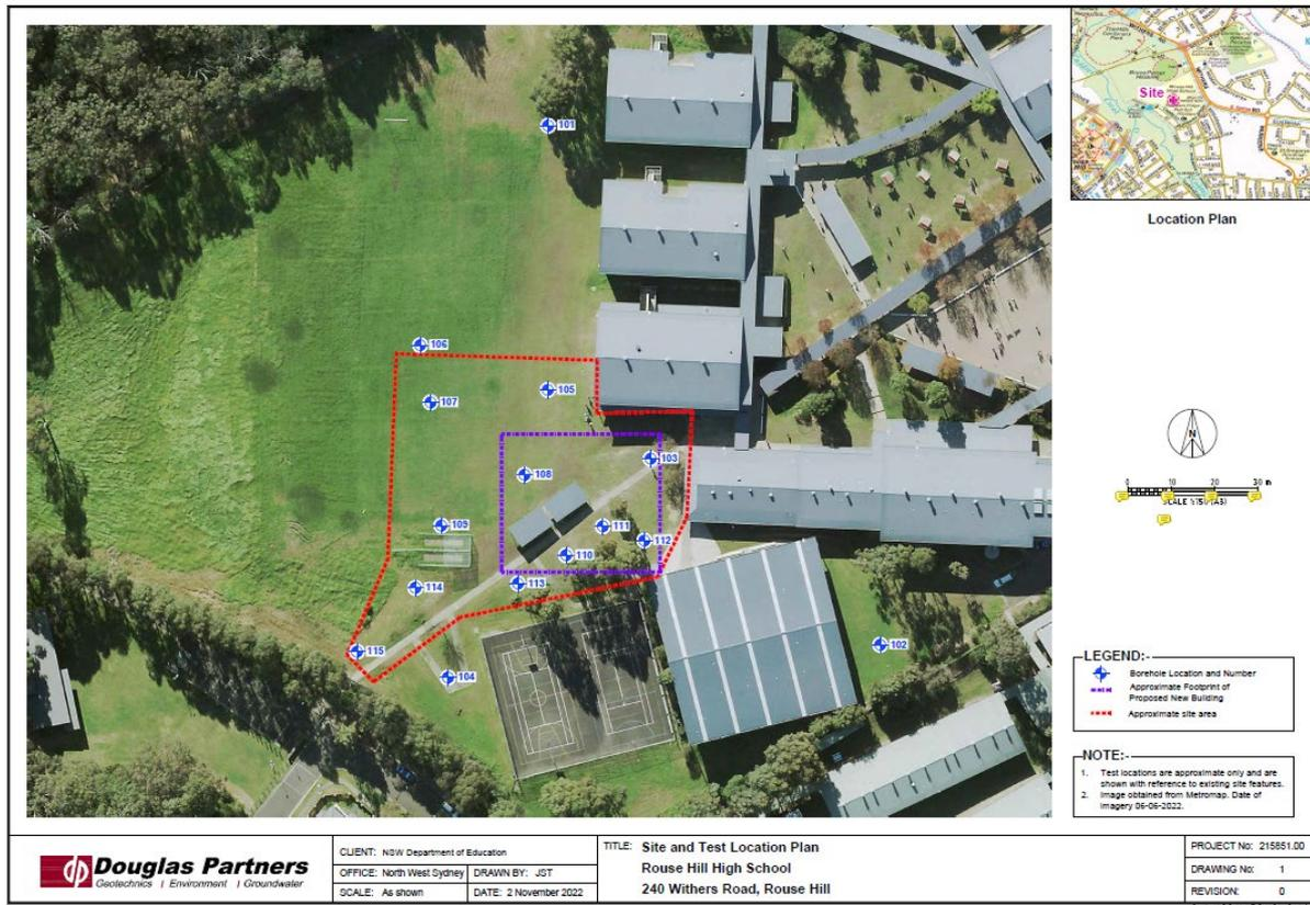
Figure 2 Douglas Partners’ borehole locations. The current program of soil sampling aims to clarify the nature and extent of topsoil/fill layers. (Source: Douglas Partners 2022)
