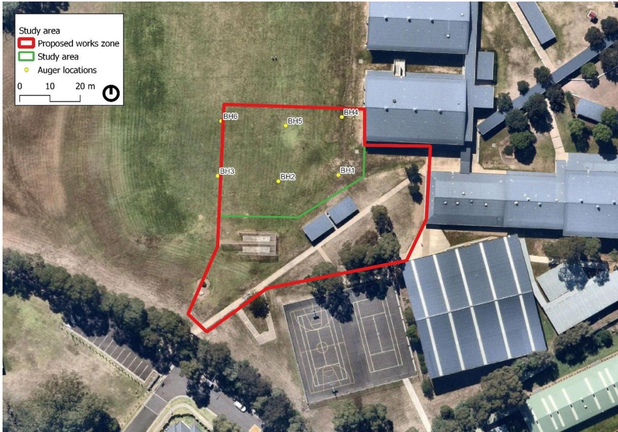
Figure 3 The locations of the six hand augers within the proposed works zone (red line) and study area (green line)—the western sports field. (Source: Nearmap 2024 with GML additions)
